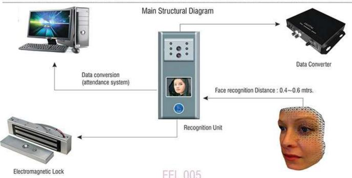
Face Recognition Touchscreen Unit - Works in Synchronisation with Electromagnetic Lock,
